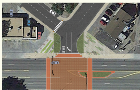
< A second phase of improvements on G St could include traffic signals or flashing pedestrian crossings, as well as pavement markings to increase safety, calm traffic, and better facilitate turning traffic.
