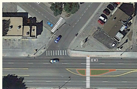
< The left image is an example of what G St could look like after an initial phase of low-cost improvements. Installing crosswalks and a short pedestrian refuge island greatly increases pedestrian safety and walkability.
