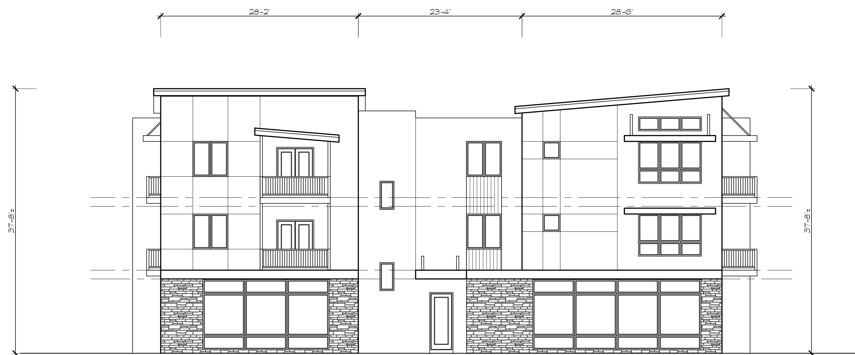
2 WEST ELEVATION BUILDING A 1/8" = 1'-0"
